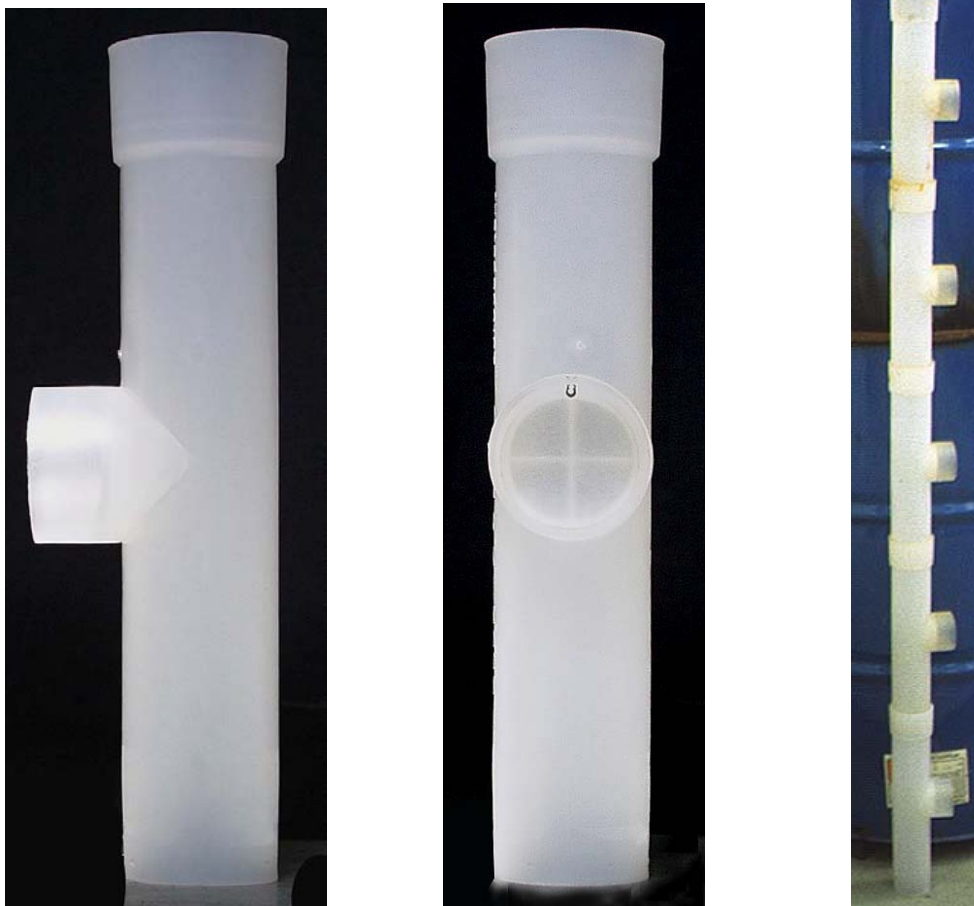
Fig. 6. Photos of a SOLVIS stratification inlet pipe and (right) 5 compound inlet pipes.
