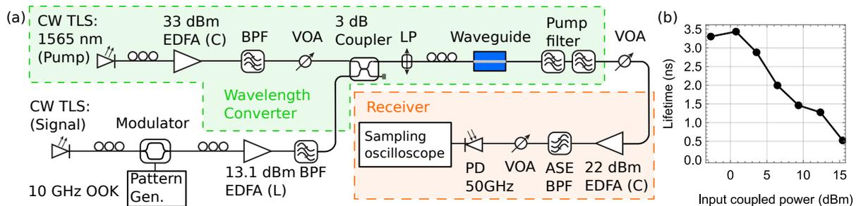
Fig. 1: (a) Experimental setup. ASE: Amplified spontaneous emission. BPF: Bandpass filter. CW: Continuous wave. EDFA: Erbium-doped fiber amplifier. LP: Linear polarizer. OOK: On-off keying. PD: Photodiode. TLS: Tunable laser source. VOA: Variable optical attenuator. (b) Measured free-carrier lifetime versus input coupled continuous-wave pump power at a wavelength of 1550 nm.
