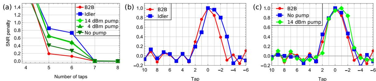
Fig. 2: (a) SNR penalty for varying number of equalizer taps. (b) Impulse responses from equalizer. Amplitudes are normalized by pulse power. Comparing back-to-back and idler. (c) Comparing back-to-back and signal.
