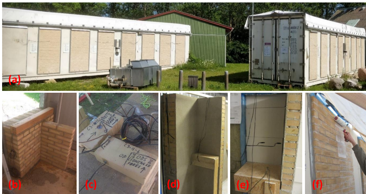
Figure 2 The experimental setup: (a): The test containers, (b): installation of the embedded wooden wall plate, (c): installation of sensors in the masonry bricks, (d): installation of the embedded wooden beam end, (e): the internal insulation with embedded sensors, (f): external treatment with hydrophobising cream. Source: Tommy Riviere Odgaard.
