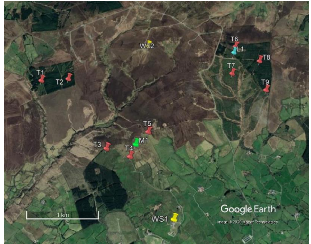
Scanning LiDAR (WS1 and WS2), met mast (M1) and vertical LiDAR (L1) deployment locations for the planned campaign.
