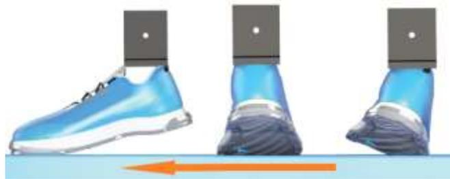
**Fig. 1** Test setups, from left to right: anterior-posterior, medio-lateral, lateral edge. The arrow indicates the movement direction of the surface (hydraulic force plate).
