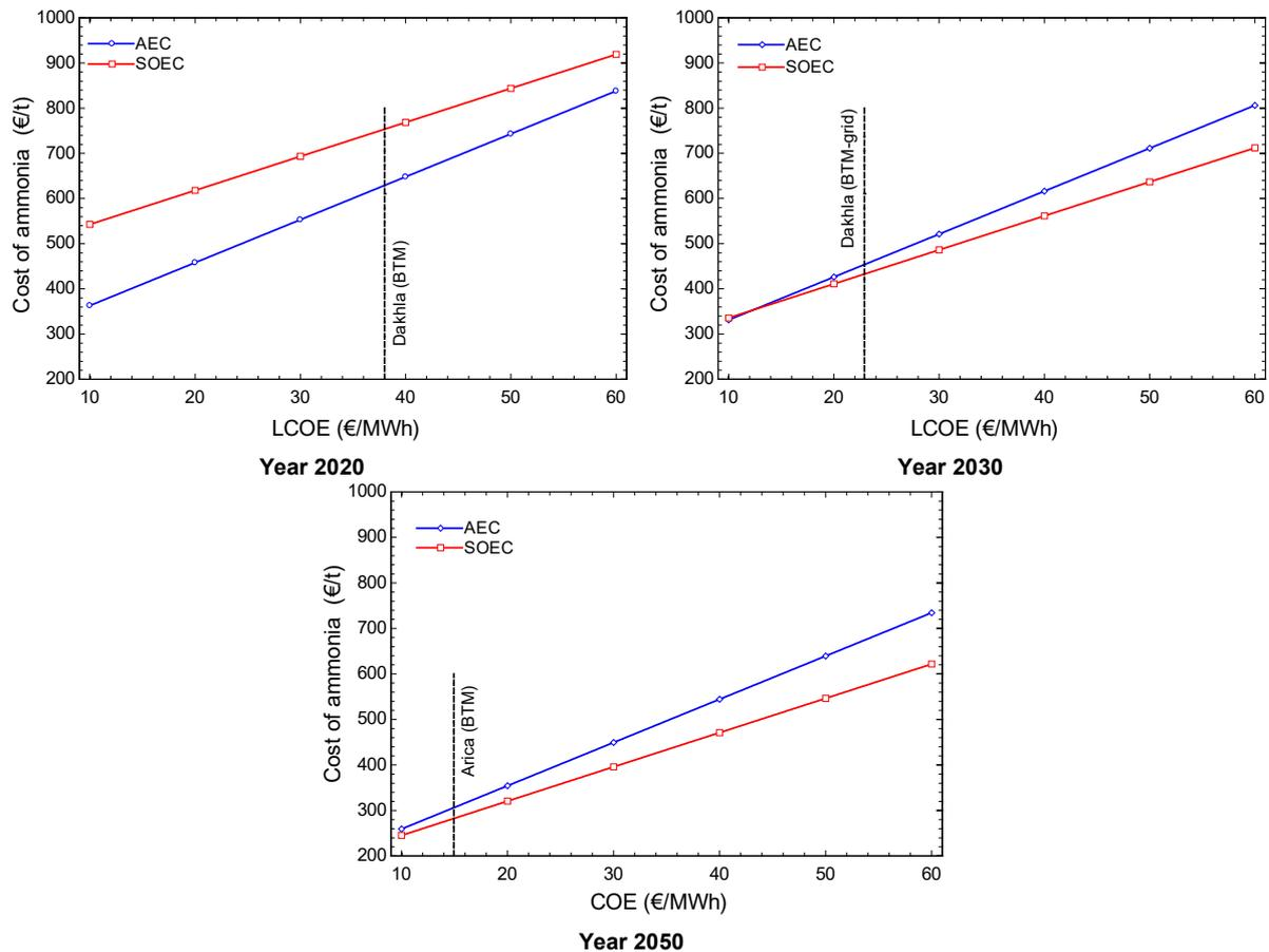
**Figure 1: Estimated cost of green ammonia from a fully flexible plant operating 7884 hours a year as a function of the levelized cost of electricity.**
