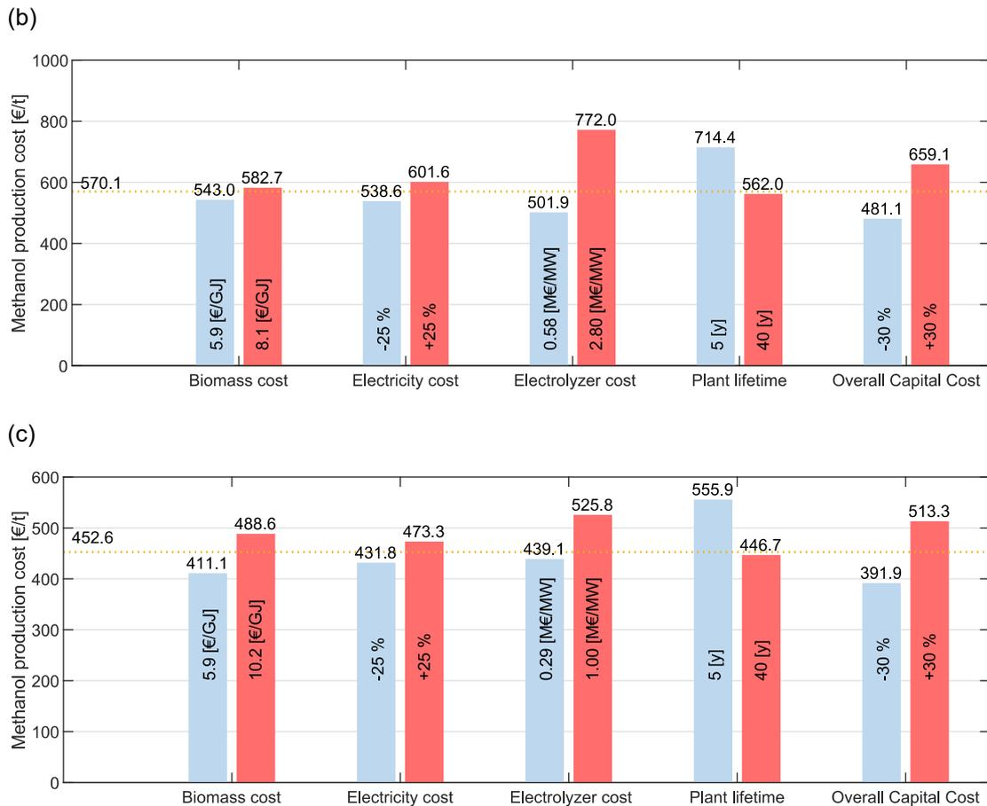
**Figure 3: Illustration of the sensitivity of the methanol cost on various of the cost driving parameters under assumptions relevant for 2020 (a), 2030 (b) and 2050 (c). The base case is with the assumptions providing the cheapest fuel in 2020, 2030 and 2050 (725 €/t, 570 €/t and 453 €/t, respectively).**
