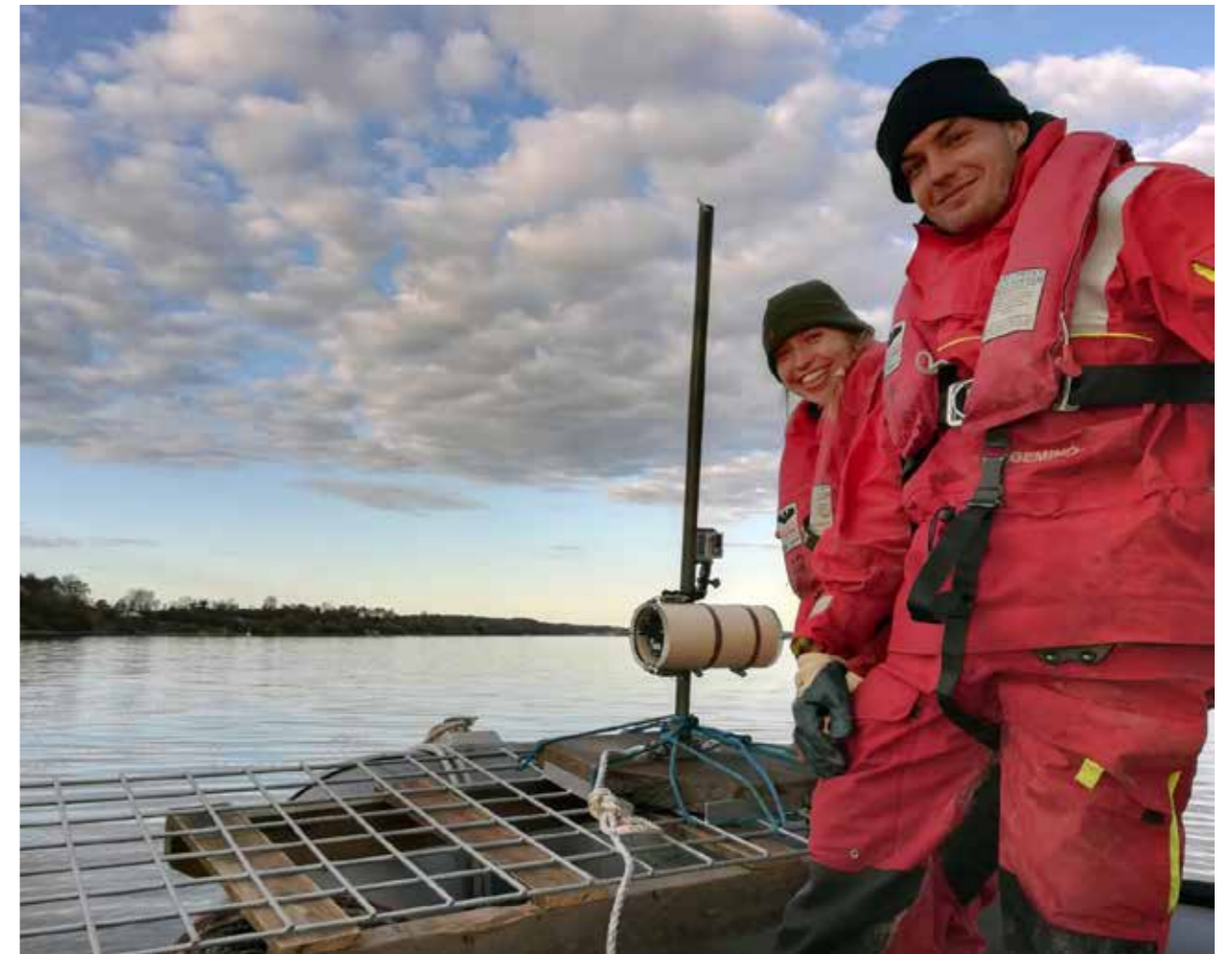
↓ Figure 5: Camera setup used for sampling in Sønderborg Bay in Spring 2021. Fieldwork activities include changing camera SD cards and the batteries every day at sea.
