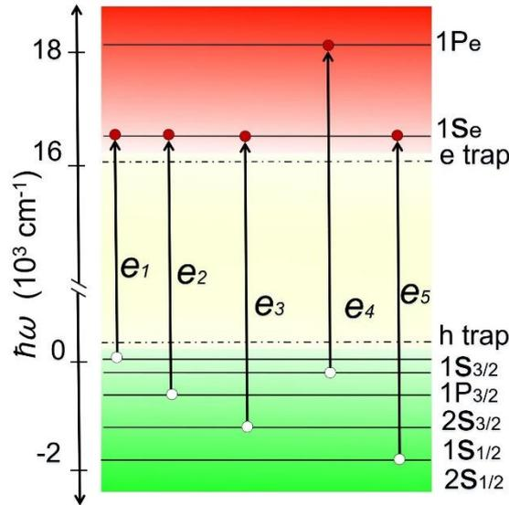
**Figure S3.** The excited states  $e_1$ ,  $e_2$ ,  $e_3$ ,  $e_4$ , and  $e_5$  in CdSe QDs.
