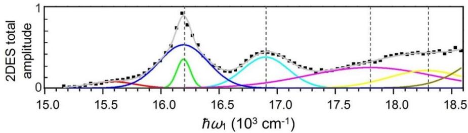
**Figure S1.** Fitting in the low-energy region of the excited states of CdSe QDs from the amplitude part of the total 2D spectrum at  $t_2 = 10\text{ ps}$  and  $\hbar\omega_3 = 16200\text{ cm}^{-1}$ , divided by the laser spectrum, as shown in our previous work<sup>1</sup>. The data (black squares) are fitted as a sum (gray line) of Gaussians corresponding to specific states (colored lines, average energies are marked by vertical dashed lines).
