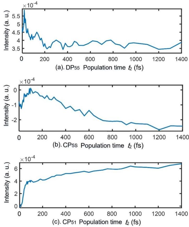
**Figure S6.** The intensities of DP<sub>55</sub>, CP<sub>55</sub>, and CP<sub>51</sub> from the real part of the rephasing 2D spectrum.
