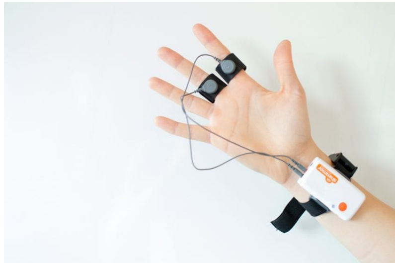
Figure 8: Shimmer3 GSR+ Unit sensor positioned to the palmar surface of the second and third finger
