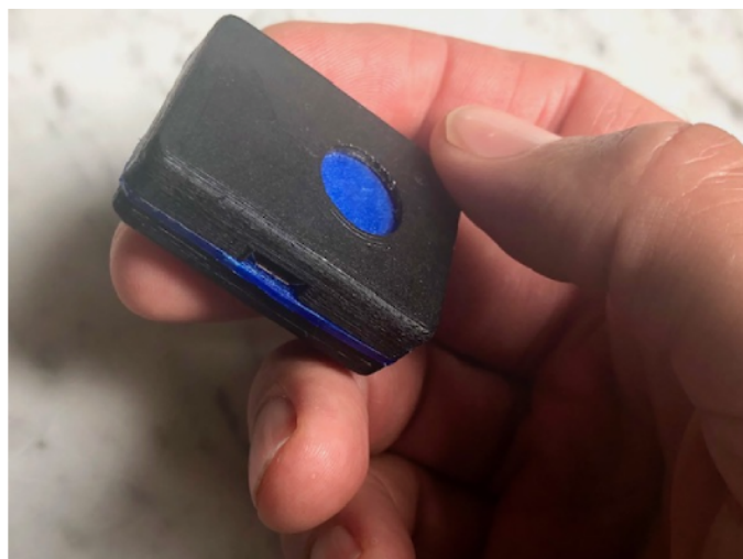
Figure 1. One Button Tracker. It is a data acquisition instrument in a 3D printed plastic casing that can be charged via a USB port. It was designed to track any subjectively experienced phenomenon.
