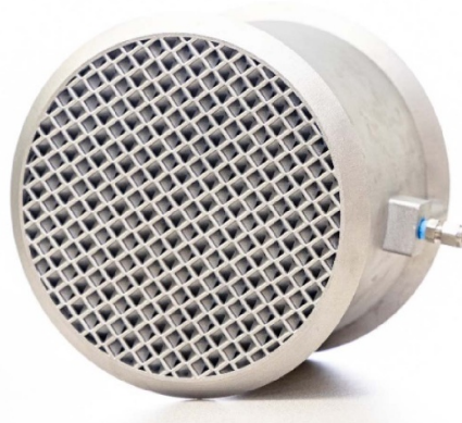
Figure 17. Intensified packing device manufactured at ORNL's manufacturing demonstration facility. This device was printed with a Concept Laser XLine 2000 laser powder bed additive manufacturing system (SLS). The material was aluminium AlSi10Mg. The ORNL intensified packing device can be used to enhance mass transfer and chemical reaction and also remove heat generated by the reaction of CO 2 with the solvent.
