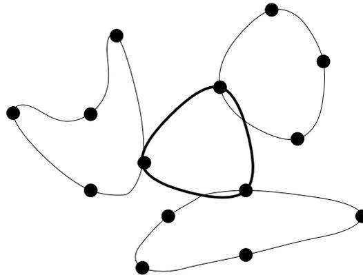
Figure 1: *An example of a hierarchical ring network.*
