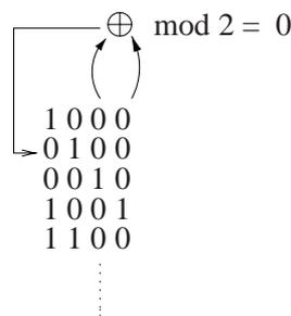
Fig. 2: Generation of a PRBS sequence, exemplified using a shift register circuit with  $n = 4$ . In the first step a zero is generated ( $0+0 \text{ mod } 2 = 0$ ). The generated number is put back in the shift register. In the second step a new zero is generated ( $0+0 \text{ mod } 2 = 0$ ) followed by a one in the next step ( $1+0 \text{ mod } 2 = 1$ ) etc.
