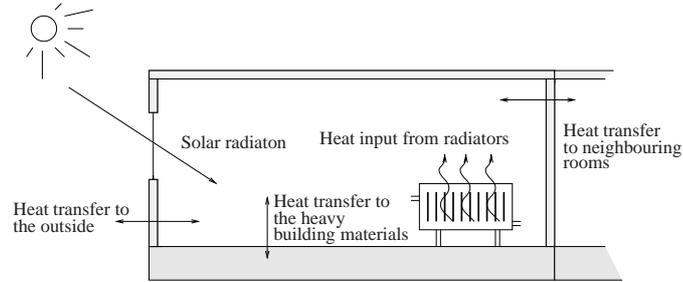
Fig. 7: A sketch of the heat transfer in the test house. The arrows symbolize the heat transfer that is assumed to be most important for the heat dynamics.
