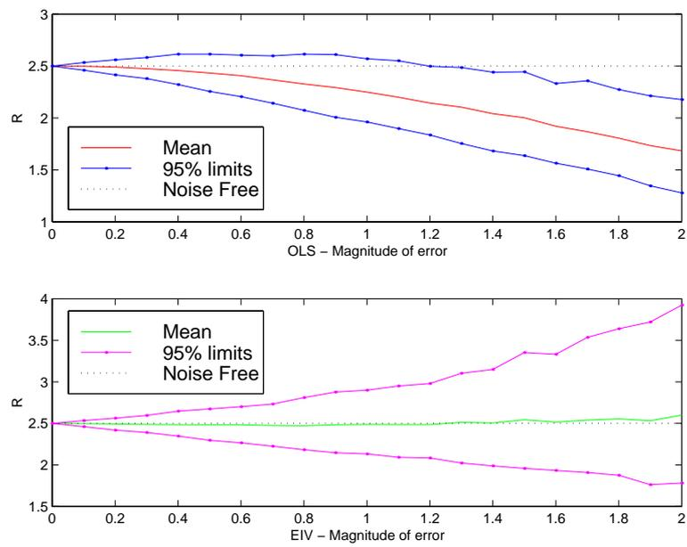
Fig. 4: Comparison of OLS (top) and EIV (bottom) estimates of the heat exchanger thermal resistance.
