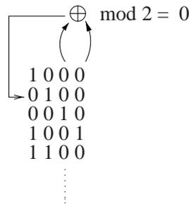
Figure 2.3: Generation of a PRBS sequence, exemplified using a shift register circuit with  $n = 4$ . In the first step a zero is generated ( $0+0 \text{ mod } 2 = 0$ ). The generated number is put back in the shift register. In the second step, a new zero is generated ( $0+0 \text{ mod } 2 = 0$ ) followed by a one in the next step ( $1+0 \text{ mod } 2 = 1$ ) etc.
