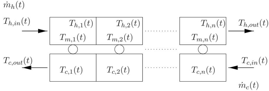
Fig. 5: The compartmental counter flow heat exchanger model.
