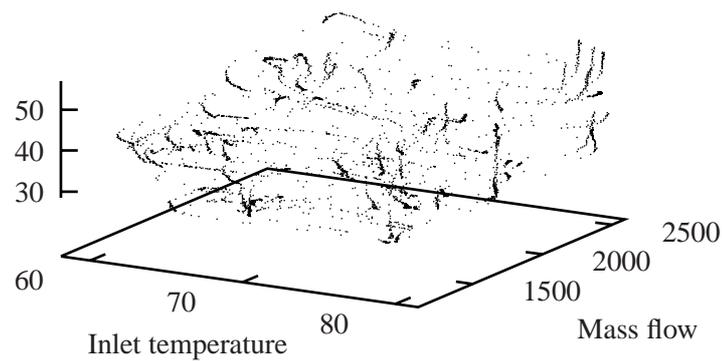
Fig. 4: Distribution of the outlet temperature as a function of the inlet temperature and the mass flow (hot side).
