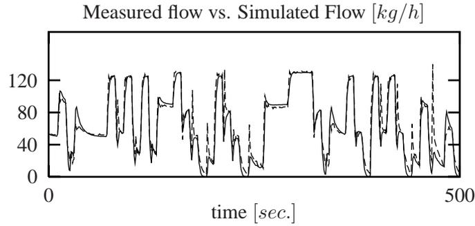
Fig. 9: Cross validation. The model is used to simulate the system using a stochastic independent time series. Simulated (solid line) and measured (dotted line).
