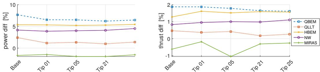
**Figure 6.** Influence of the SmartTip extension on the aerodyn. power and thrust in reference to the corresponding CFD solution at  $8 \text{ ms}^{-1}$  wind speed
