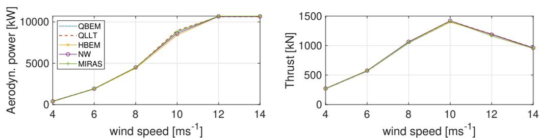
**Figure 7.** Aerodyn. power and thrust of the baseline rotor, aeroelastic load case
