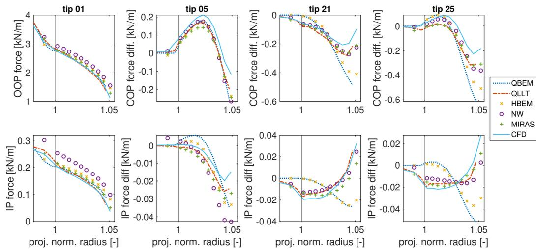
**Figure 5.** Distributed in- and out-of-plane loads along tip 01 and the difference in loads to tip 01 at  $8 \text{ ms}^{-1}$  wind speed. The vertical line marks the beginning of the extension
