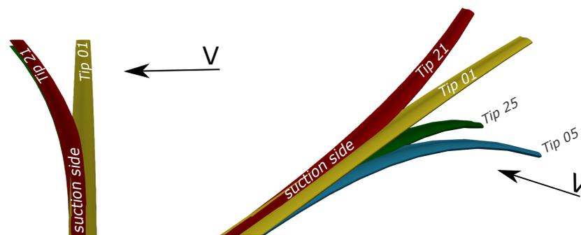
**Figure 1.** SmartTip extensions, tip 01 - extension, tip 05 - downwind dihedral, tip 21 - backwards sweep and tip 25 - sweep and dihedral
