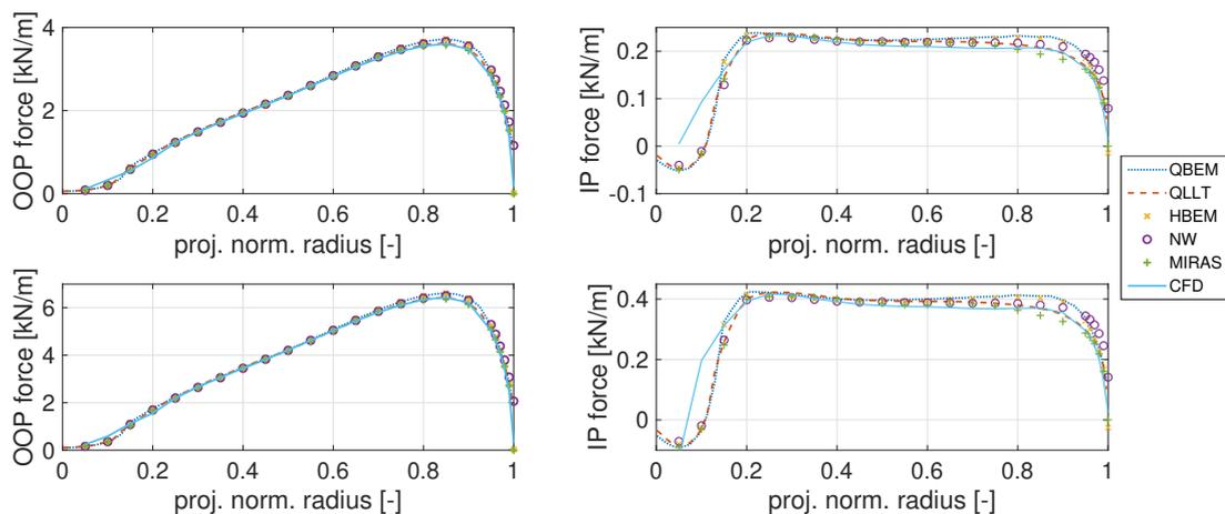
**Figure 4.** Distributed loads on the baseline rotor at  $6 \text{ ms}^{-1}$  (top) and  $8 \text{ ms}^{-1}$  (bottom) wind speed
