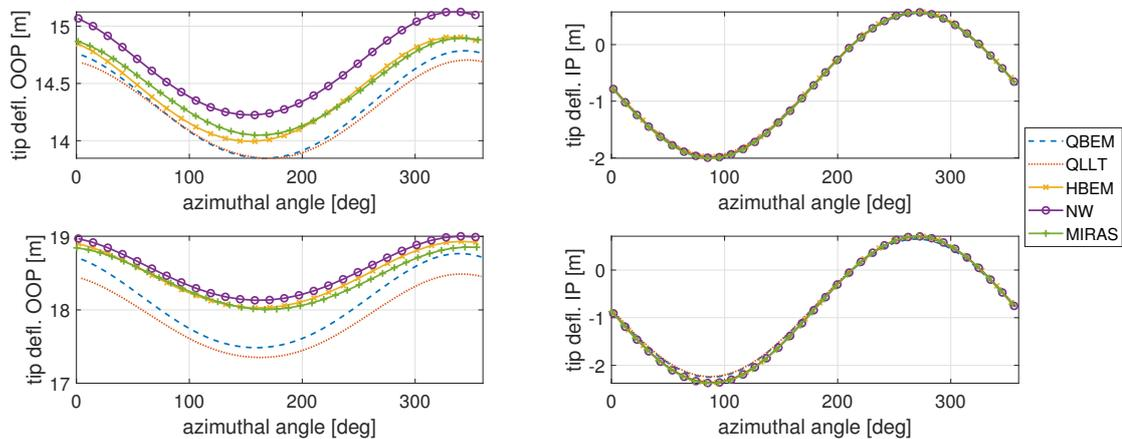
**Figure 9.** Tip deflections in out-of-plane and in-plane direction at  $10 \text{ ms}^{-1}$  wind speed. Baseline (top), swept rotor (bottom)
