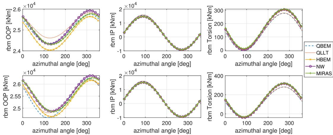
**Figure 8.** Root bending moments (at  $r = 2.89$  m) in the out-of-plane, in-plane and torsional DOF at  $10 \text{ ms}^{-1}$  wind speed. Baseline (top), swept rotor (bottom)
