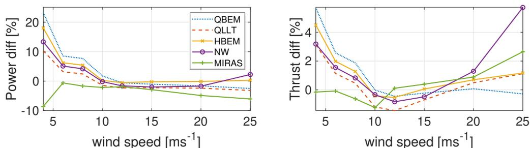
**Figure 3.** Relative power and thrust difference in reference to the CFD power curve
