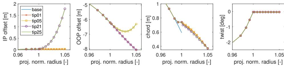
**Figure 2.** Geometric properties of the SmartTip extensions
