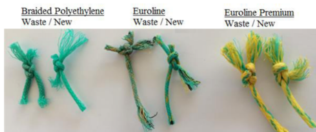
Figure 2. Waste and new PE fishing nets from Euronete, used for characterisation of the mechanical properties of single fibres. Braided polyethylene (BP), Euroline (EU), and Euroline premium (EP).
