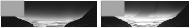
Fig. 1. (a) Normal process with homogeneous intensity on polycrystalline surface. (b) abnormal process with watermarks on polycrystalline surface.
