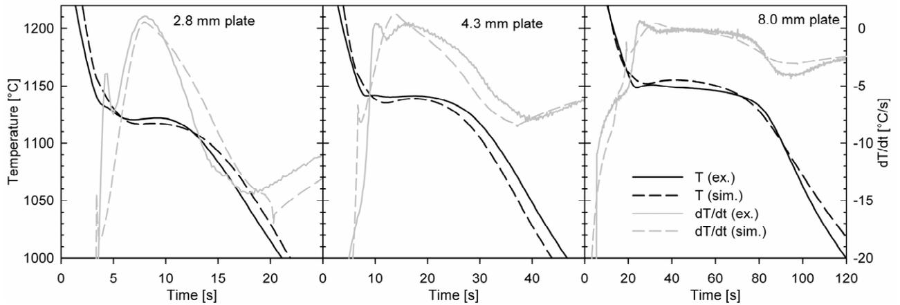
Fig. 8 Experimental and simulated temperature and dT/dt curves for the the three different plate thicknesses for casting E.
