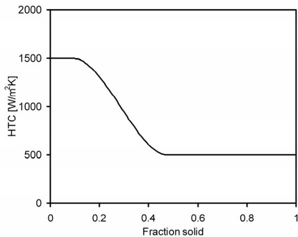
Fig. 6 HTC as a function of the solid fraction in the surface of the casting next to the mould
