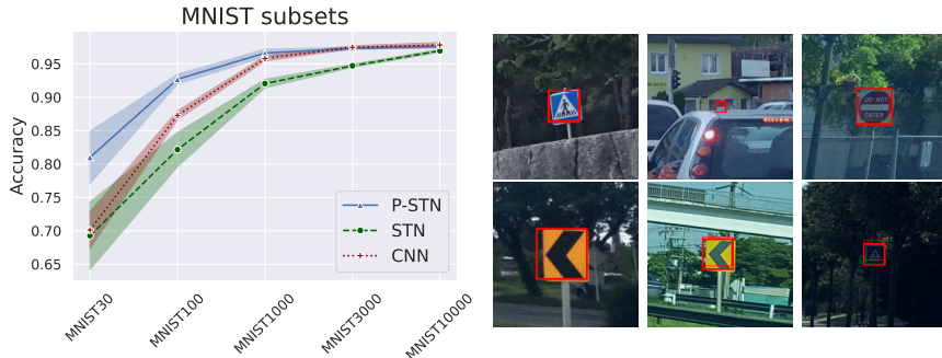
Figure 4.6: Left: Performances of P-STN, STN and CNN on MNIST subsets (mean \pm one STD across five folds). Right: The P-STN learns to localise traffic signs in the challenging MTSD dataset. 10 sampled transformations are shown with their corresponding bounding boxes overlaid, here on test data. The learned variations improve performance on the downstream classification task. Figure from Paper 2.
