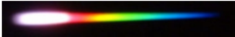
Figure 4.13: The spectrum from Figure 4.12 visualized by sending it through a prism. Experiment by Erling Riis, Strathclyde university, Glasgow. Kindly borrowed from Crystal Fibre A/S. Courtesy NKT Research.
