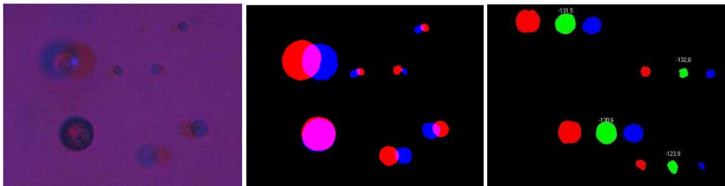
**Figure 2:** Stereoscopic images of an assembly of trapped beads of various sizes. Second image shows image analysis of the first actual image. The last image shows how the analyzed image looks when a centered green illumination is added to the illumination seen in Fig. 1.
