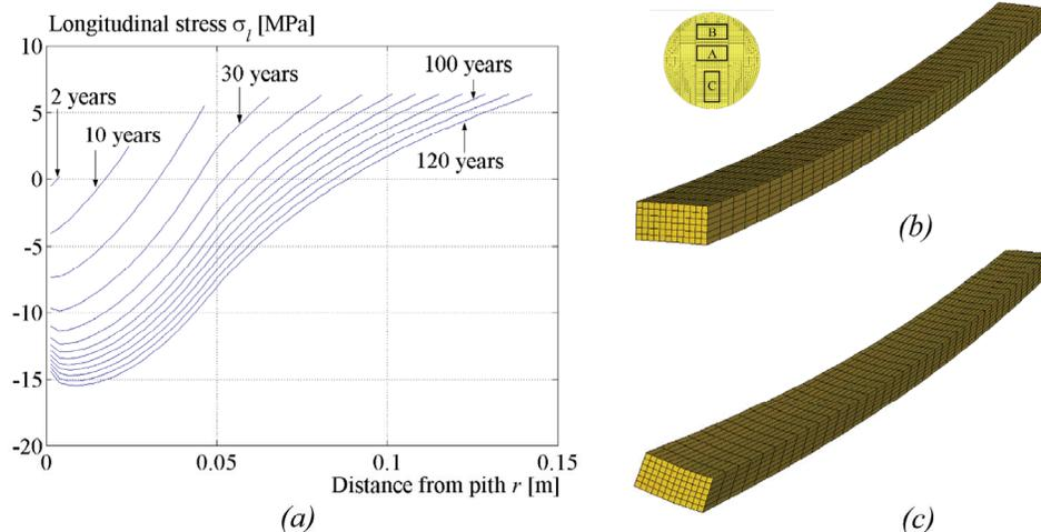
**Figure 1:** Growth stresses and distortion of board A (def. are magnified by factor of 3), (a) longitudinal stress profiles during 120 years for a tree with good growth condition (b) distortion after sawing (bow), (c) distortion after drying (both twist and bow).
