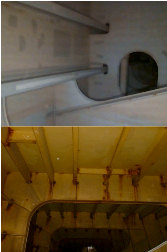
Fig. 1. Two vessels of the same type, but with different age. On the top is a younger vessel and on the bottom is an older vessel. Note the difference in color as the coating degrades; from gray-toned to yellow-toned. (For interpretation of the references to color in this figure legend, the reader is referred to the web version of this article.)
