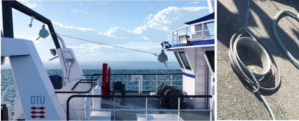
Figure 6. The coax cable and winch onboard the DTU research vessel (left) and the tension release ring (right).
