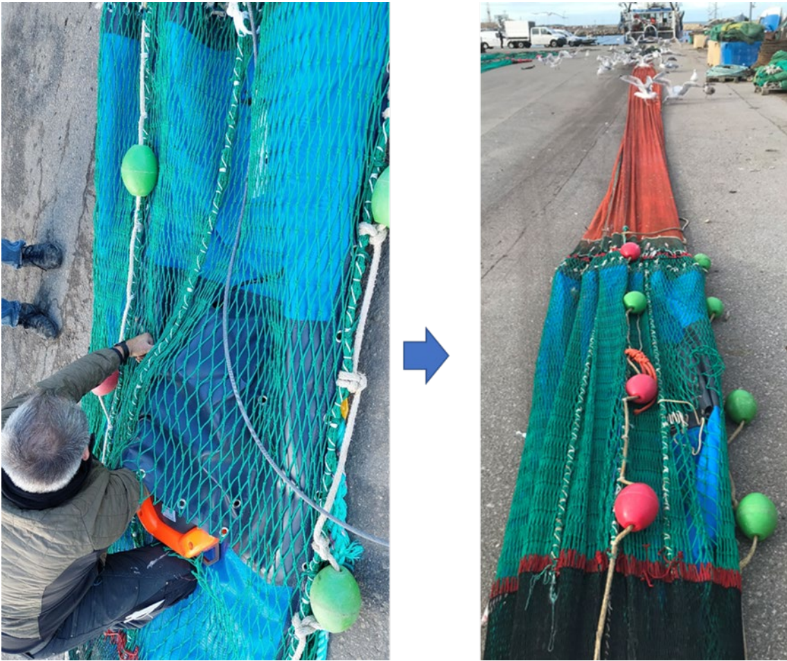
Figure 15. Mounting of camera and connecting transmission and power cable in deepwater shrimp trawl (left). Camera system mounted and ready to go at sea (right).
