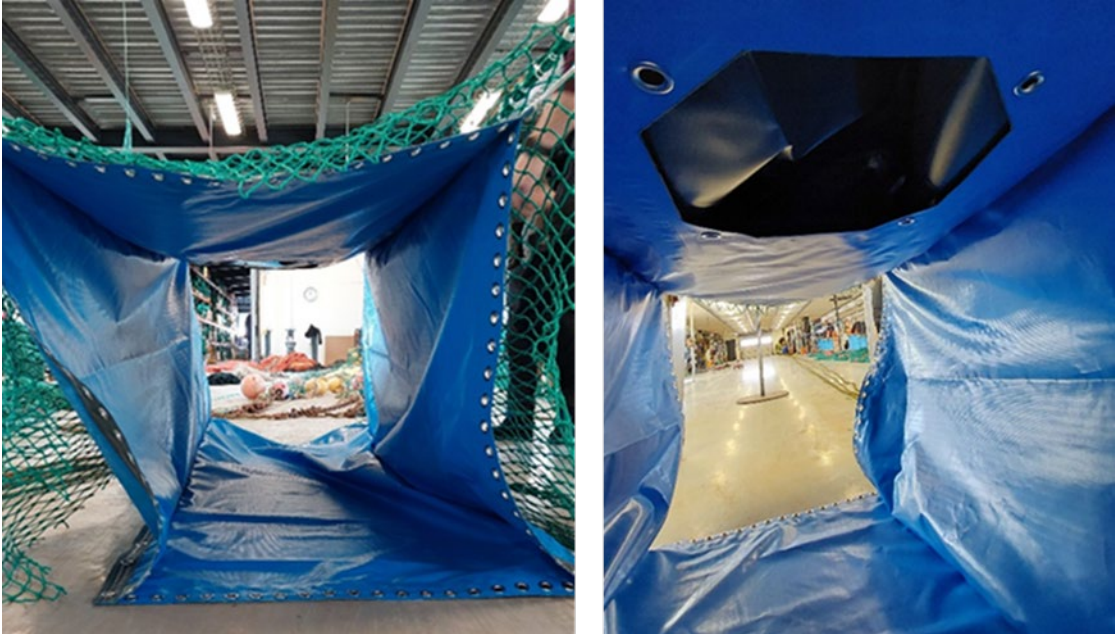
Figure 14. Observation section for deepwater shrimp fisheries. The observation scene is inserted in a 3.5m four panel netting section (left). Camera pocket on the inside (right).
