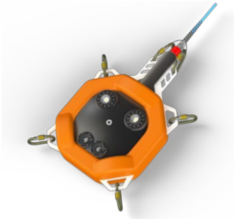
Figure 2. The camera (SeaScout), here in a stereo setup, and LED light source compacted in a waterproof case.
