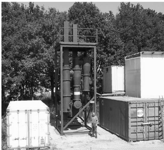
**Figure 3:** The 500 kW LT-CFB test plant at DTU
