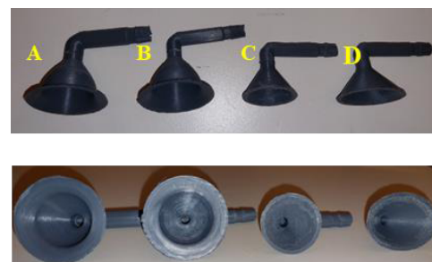
Fig.3 Pictures of the four nozzle designs: A. flanged nozzle with inner Ø8 mm, B. flanged nozzle with inner Ø6 mm, C. circular nozzle with inner Ø6 mm, D. Oval nozzle with inner Ø6 mm.
