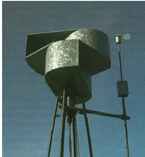
Figure 33: Drag-driven vertical wind turbine (Savonius type)
