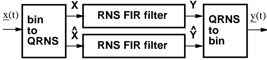
Figure 3.20: Structure of QRNS filter.
