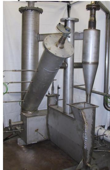
Figure 9: 100 kW Laboratory gasifier (Before insulation)
