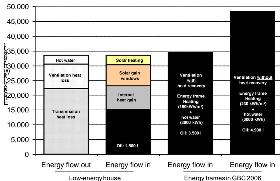
Figure 3. Energy balance of the 197 m<sup>2</sup> low-energy house compared with the demands of the Greenlandic building code.
