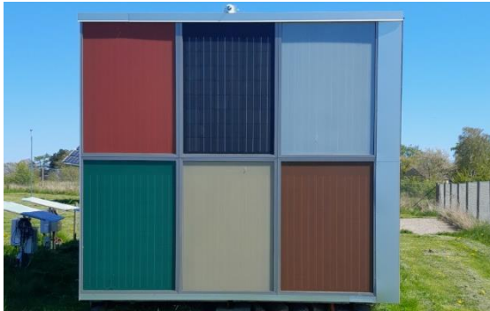
Figure 1: West-facing BIPV façade featuring five colored modules and one uncolored reference.
