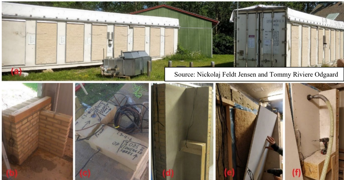
Figure 1. The experimental setup. (a): Test containers. (b) Embedded wooden wall plates. (c) Sensors in masonry bricks. (d) Embedded wooden beam ends. (e) Hemp insulation, and (f) Cellulose insulation being installed.
