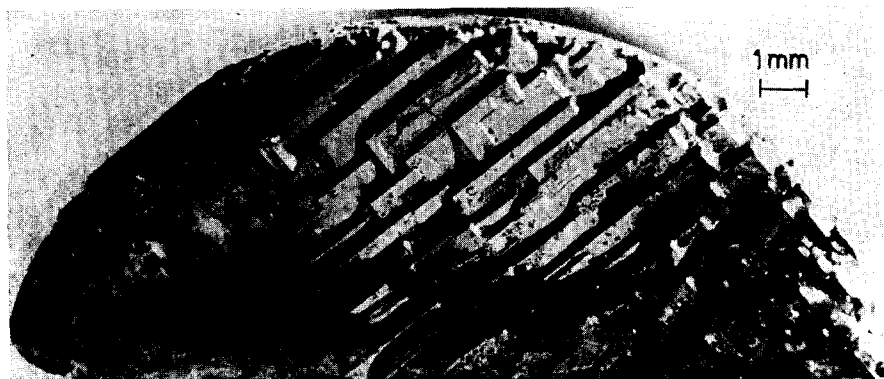
FIG. 1. Layered structure of the decanted interface of a \text{Bi}_{0.86}\text{Sb}_{0.15} alloy single crystal. The plane of the view shown here is perpendicular to the axis of the ingot. X-ray analyses showed that the facets are {100} planes.
