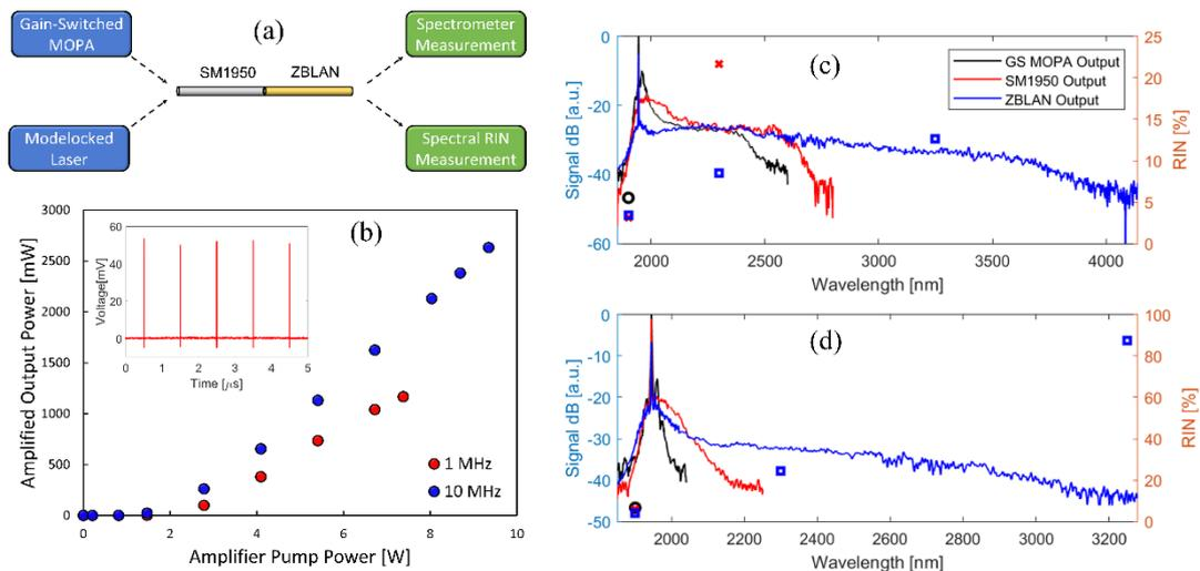
**Fig. 1** Experimental schematic (a), gain-switched output power at 1 MHz and 10 MHz with 1 MHz pulse train example (inset) (b), output spectrum and RIN from gain-switched system, SM1950 and ZBLAN at 1 MHz (c) and 10 MHz (d).
