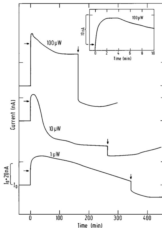
FIG. 4. The figure shows PC and PPC for one sample obtained with three different illumination intensities of a 544 nm wavelength. The horizontal arrows at time  $t=0$  indicate the heights of the prompt increases in PC and the vertical arrows indicate the time at which the illumination was switched off. The insert shows the evolution of the curve obtained with illumination power equal to  $100 \mu\text{W}$ , during the first 10 min of illumination.
