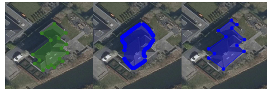
Figure 1. The aim of our study is to predict the most compact set of vertices that produce a geometrically accurate building delineation from data acquired under real-world conditions. From left to right: Ground truth, HiSup [22], GAST (ours).
