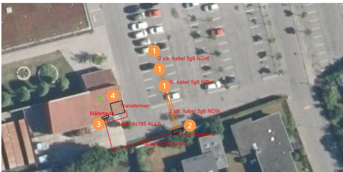
Figure 10: Overview of the parking lot. 1) Location of chargers. Each location marked with “1” will host two chargers, on opposite sites; 2) Cable cabinet; 3) Meter cabinet; 4) Transformer.
