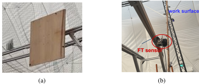
Fig. 7: Experiment setup, (a) a wooden board as work surface, (b) a FT sensor mounted behind the work surface.
