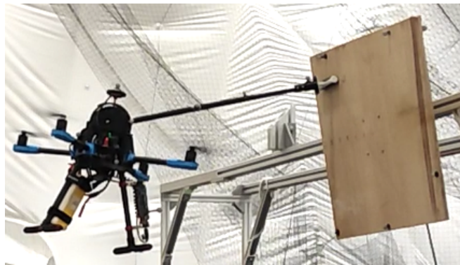
Fig. 1: A quadrotor-based aerial manipulator is pushing on a flat oriented work surface.
