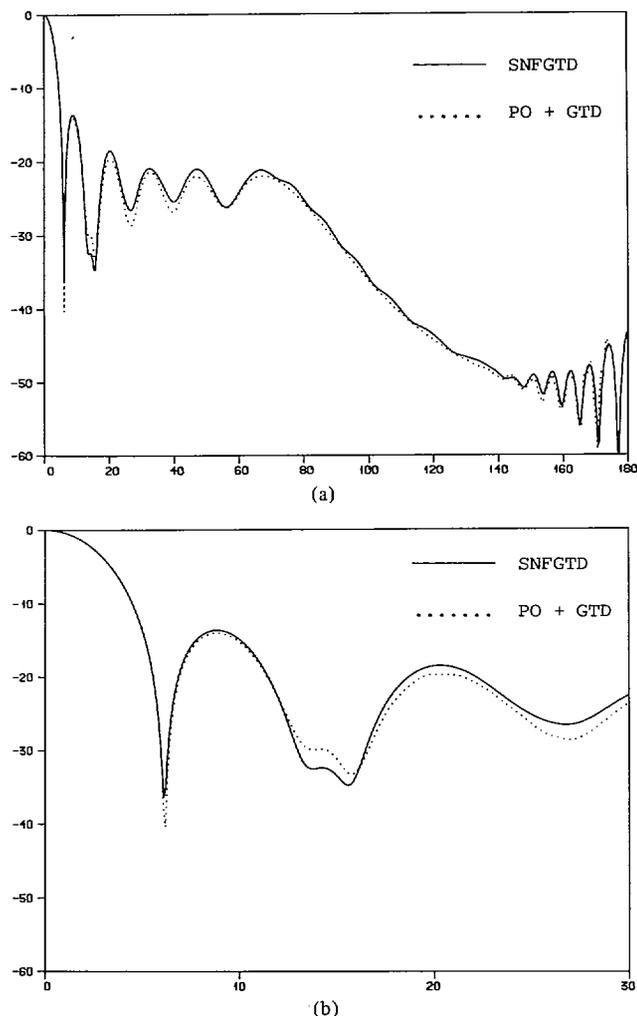
Fig. 2. (a) Comparison of SNFGTD, MM, second PO supplemented with GTD beyond  $20^\circ$  for the Afifi antenna. (b) Comparison of SNFGTD, MM, second PO supplemented with GTD beyond  $20^\circ$  for the Afifi antenna (expanded scale).
