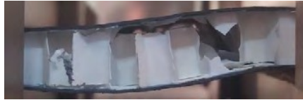
Figure 7. Core Shear Failure of PPS Sandwich
