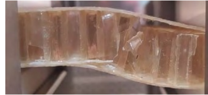
Figure 8. Core Shear Failure of PEI Sandwich
