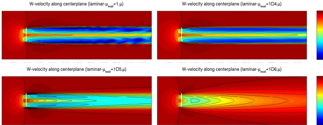
Figure 1: Axial-velocity for different molecular viscosities ( $Re = 10^8, 10^4, 10^3, 10^2$ )
