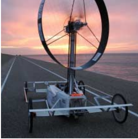
Figure 2: Example of a wind car: the WindTurbinecar [4] racing along the dike, against the wind at the 2008 Aeolus race in Den Helder, the Netherlands.
