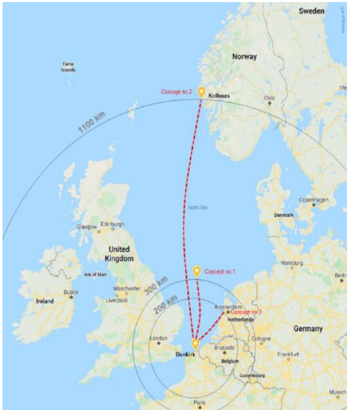
Figure 3.1: 3D project CO 2 storage concepts across the North Sea. Concepts 1 and 3 are considered for pipeline transport, while Concept 2 is evaluated for ship transport. This study exclusively focuses on the pipeline delivery of CO 2 via Concept 3.
