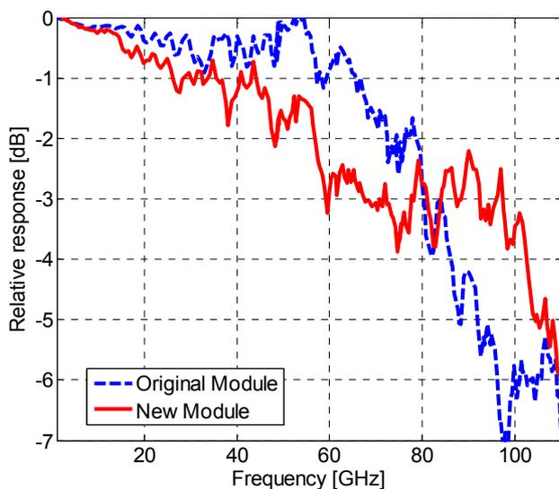
Fig. 9 Measured relative responses of the original module and the new preliminary module.
