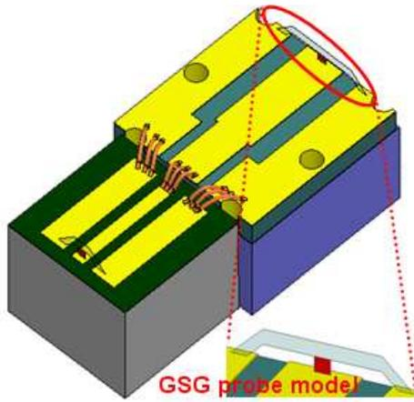
Fig. 2 An EM model of a CPW-CBCPW wire-bonding transition; the excitation structure is enlarged as an inset.
