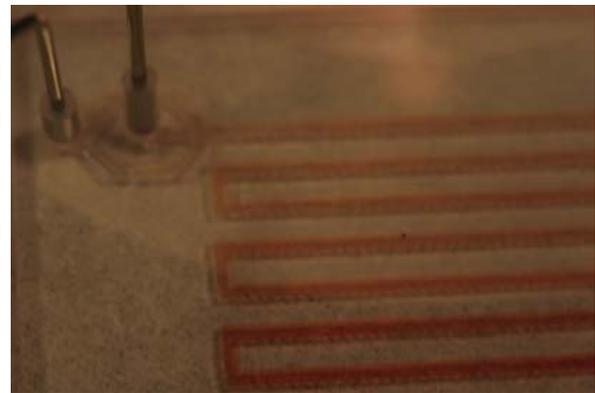
Figure 6. Interconnects: Silicon tubing and modified needles.
