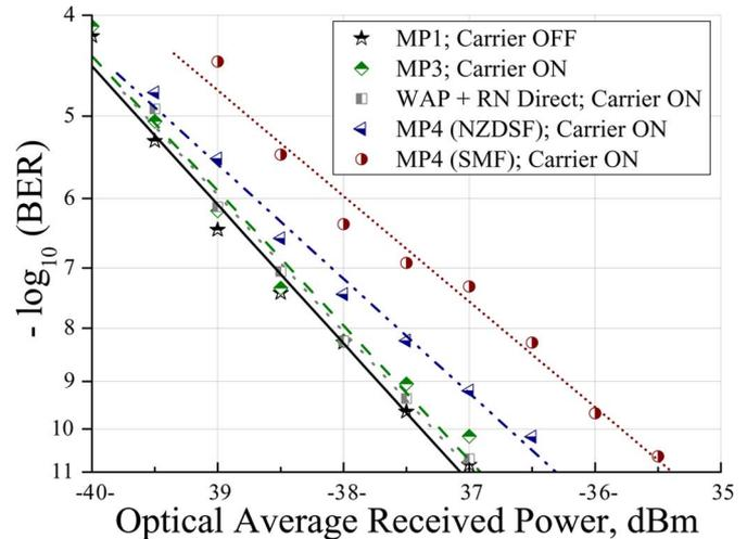
Fig. 5. Receiver sensitivity analysis of the access link system at various points, with a PRBS of length  $2^{15} - 1$ . The baseline is at measuring point (MP) 1, with the 20-GHz carrier OFF. Carrier-ON receiver sensitivity at MP2 is also presented, and also for direct connection of WAP to RN (WAP + RN) without the 20-km SMF. Results obtained at the access link output are shown for 50-km *transmission fiber* of SMF and NZDSF type.
