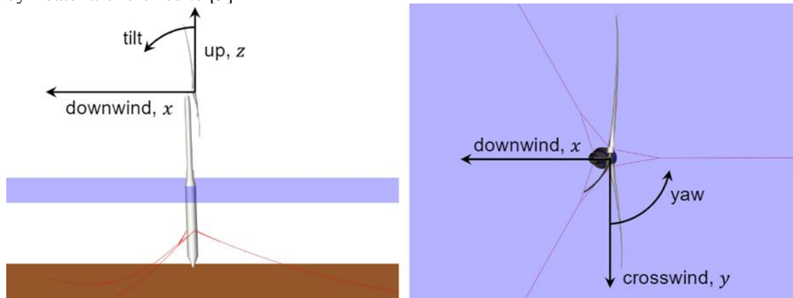
Figure 1. Selected floating offshore wind turbine (IEA 15 MW reference turbine with WindCrete spar-buoy floater) and the assumed coordinate frame [5].
