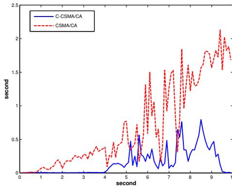
Fig. 7. Queuing delay comparison of C-CSMA/CA with CSMA/CA
