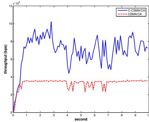
Fig. 6. Throughput comparison of C-CSMA/CA with CSMA/CA
