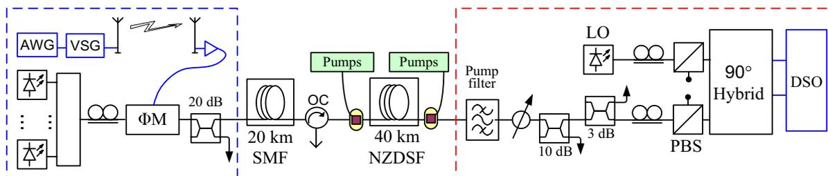
Fig. 2: Experimental setup description
