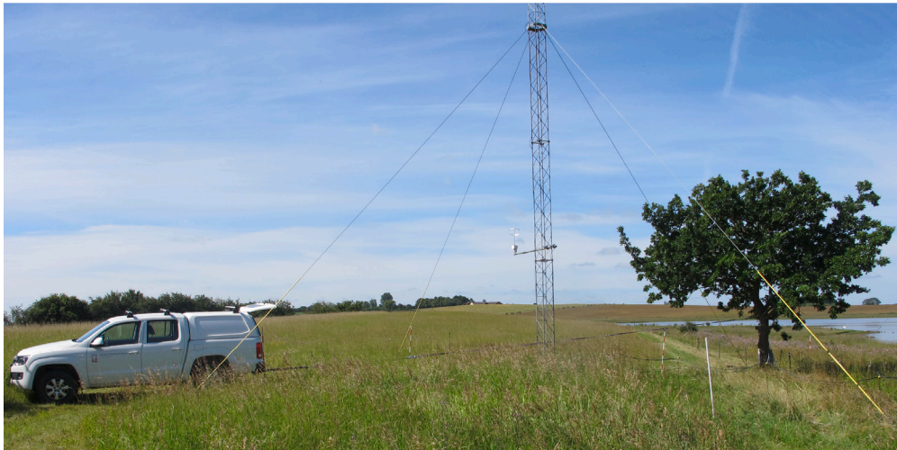
Fig. 14. Photograph of a pulling test based on a static load used to calibrate the strain gauges installed at the base of the stem of the tree. In the photograph one can see the truck used as an anchor, the steel wire used to apply a load on the tree, the oak tree and the meteorological mast used to study the wind conditions at the lee-side of the tree. At the time of this calibration, only one sonic anemometer was installed on the mast at 4 m above the ground.
