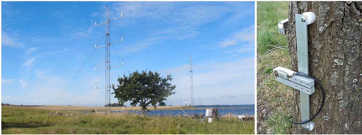
Fig. 1. Photographs of the open-grown oak tree and of the two meteorological masts used for monitoring the lee- and windward wind conditions of the tree (left) and of the caliper transducer of the strain gauge used to monitor the deformation of the stem (right).
