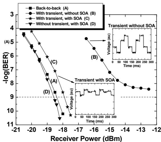
Figure 2: BER measurement results and multi-power level burst transient waveforms
